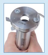
2 Thread adaptors are available in various sizes for the spark plugs that need to be set (M14, M18 or 7/8"). The adaptors can be mounted or exchanged easily with the included screws and the hex key.
