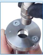
3 The integrated quick-release lock guarantees rapid changes and secure holding of the spark plugs while they are being set.
